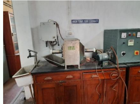
High Temperature Tube Furnace. Operable in air and Vacuum (upto 1700°C)
