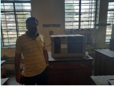
High Temperature Muffle Furnace (upto 1700°C)
