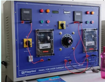
Over Current & Earth Fault Relay
