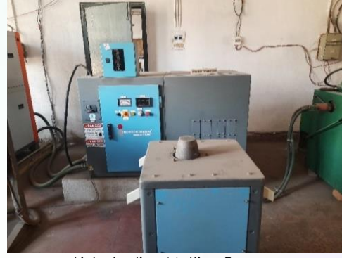
Air Induction Melting Furnace
