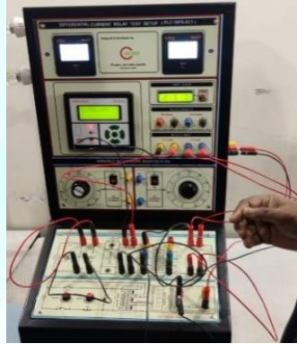
Differential Current Relay Test Setup
