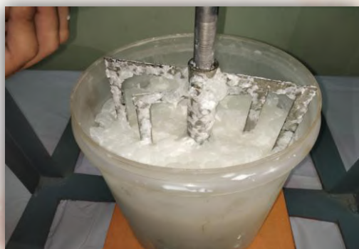
Butter churning machine with reverse rotating blades
