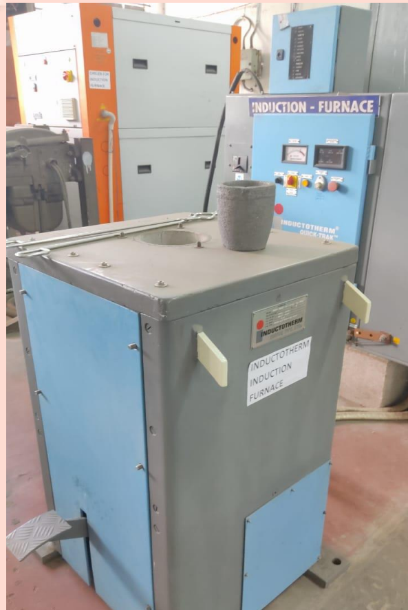
Induction Melting Furnace
