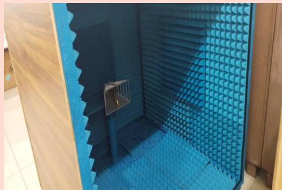
3D Antenna Radiation Pattern and Gain Measurement System with Portable Anechoic Boxes Components (Transmitter)
