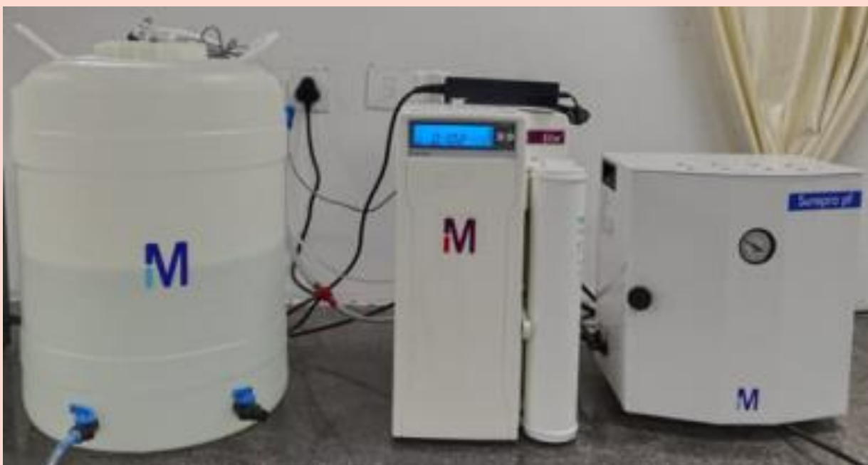
Deionised water setup unit
