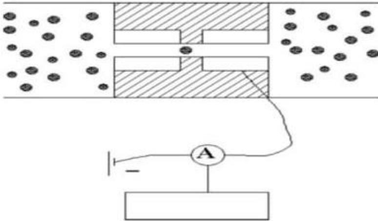
In this type of machine the powder is suspended in an electrolyte solution.
