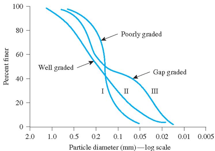
**Figure 2.27** Different types of particle-size distribution curves
