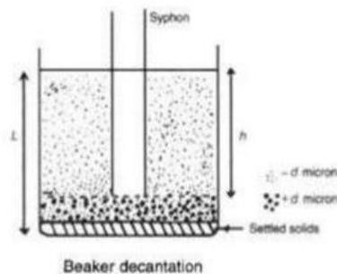
The material under test is uniformly dispersed in low concentration in water contained in a beaker. A wetting agent may need to be added to ensure complete dispersion of the particles.
