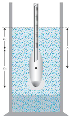
Figure 2.24 Definition of  $L$  in hydrometer test
