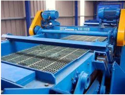
(Resonance Screens -Mac's screens)
