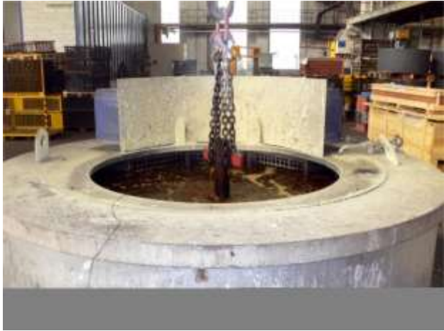
Fig 1 Salt bath I –austenitisation heat low-temperature salt-bath for isothermal
