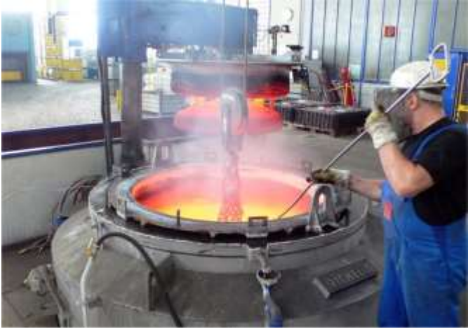
Fig 1 Salt bath I –austenitisation heat low-temperature salt-bath for isothermal
