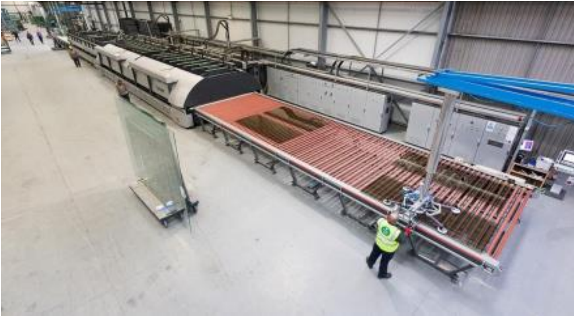
► Four glass panels on a tempering furnace at Glaston.
