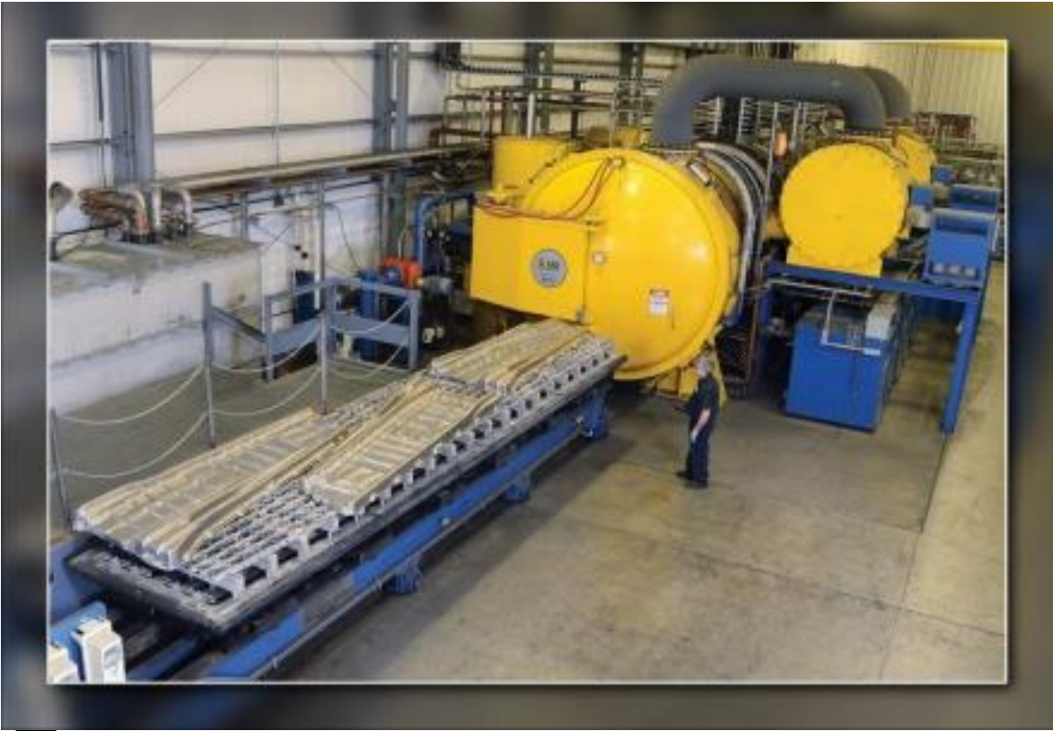
▶ A vacuum capsule used for heat treating in Embraer.
