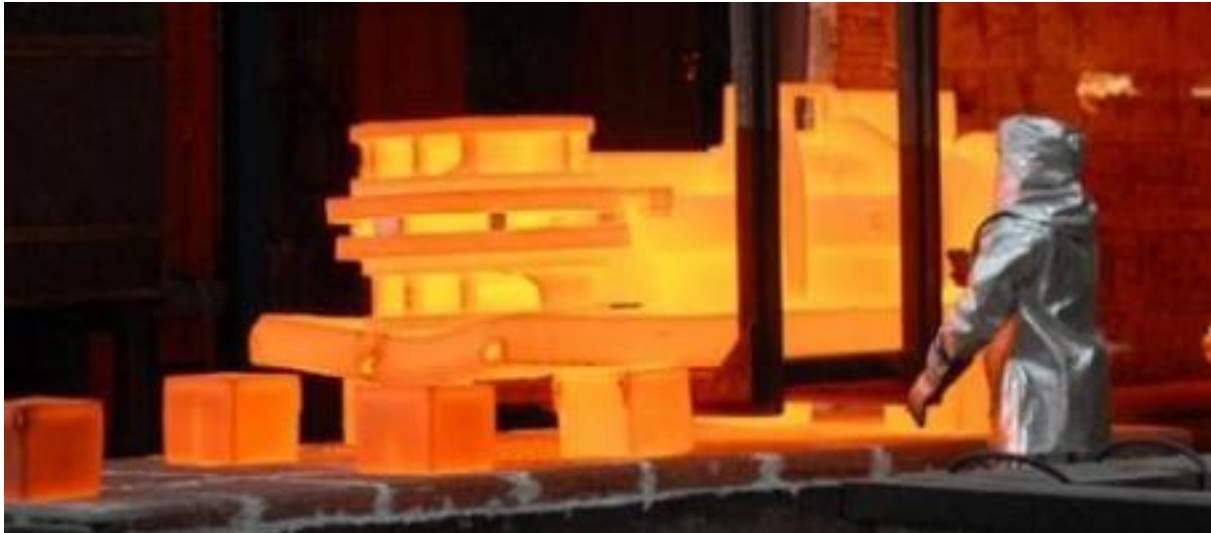
▶ Aluminium castings after post air-heating.
